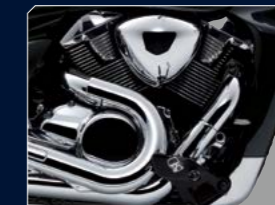
1,783cc 1 4-stroke DOHC V-twin engine
