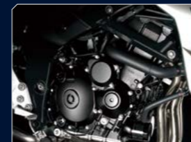
4-stroke, 4-cylinder, liquid-cooled, DOHC engine
