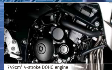
749cm 3 4-stroke DOHC engine
