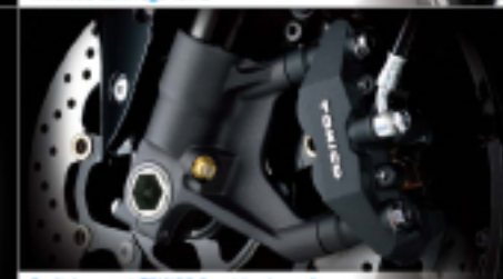
Radial-mount TORICO front brake calipers
