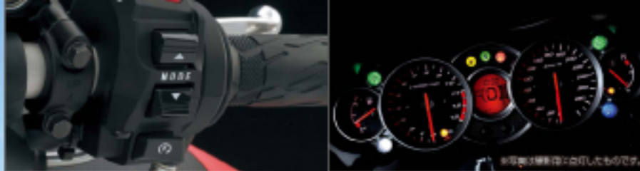
Suzuki Drive Mode Selector (S-DMS)
