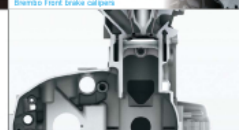
Crankcase ventilation holes
