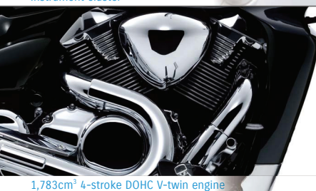
1,783cm 3 4-stroke DOHC V-twin engine
