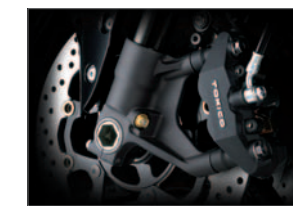
Radial-mount TOKICO front brake calipers
