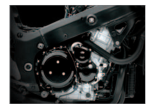
1340cm 3 4-stroke DOHC engine
