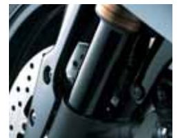
DLC-coated inner fork tubes
