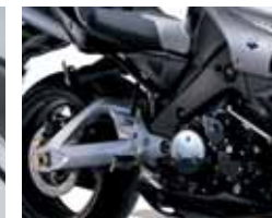
Aluminum frame and swingarm
