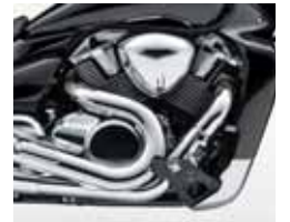
1,783cm 3 liquid-cooled 4-stroke DOHC V-twin engine
