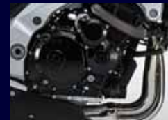
Liquid-cooled inline 4-cylinder, 4-stroke engine
